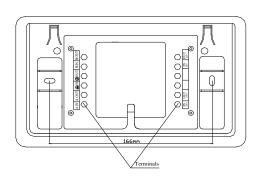
The system cables connect to the base, and linked to the repeater by internal cables.
